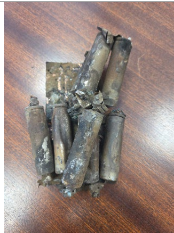
Figure 4: The remains of a li-ion battery which caused a scrap metal fire in a port.
