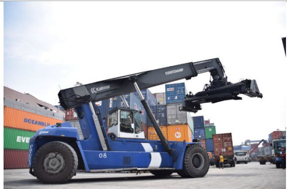
Figure 2: A battery-powered reach stacker. ©Shutterstock stock image.
