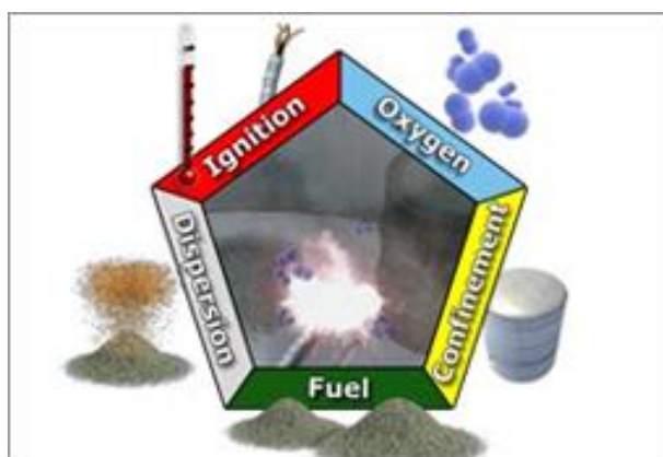
Figure 3 Explosion pentagon - conditions required for an explosion to take place
