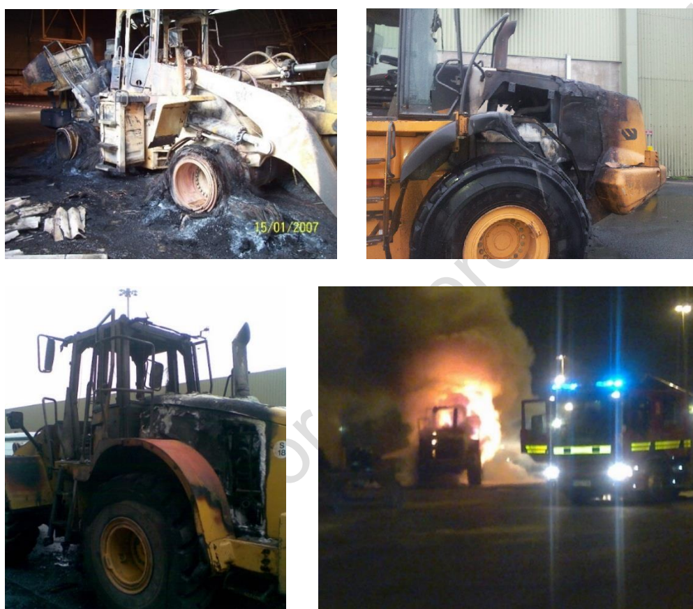
Figure 2 Examples of fire damaged handling plant
