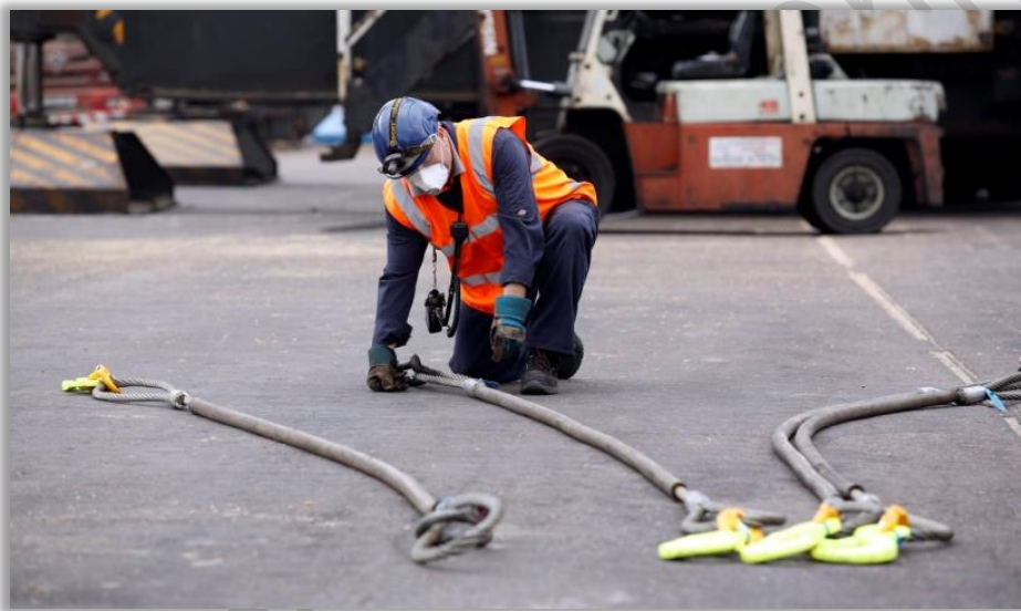
Inspection of lifting accessories prior to use
