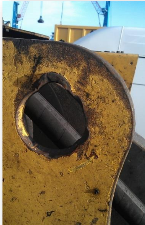
Original equipment lifting eye showing signs of deformation following multiple lifts.
