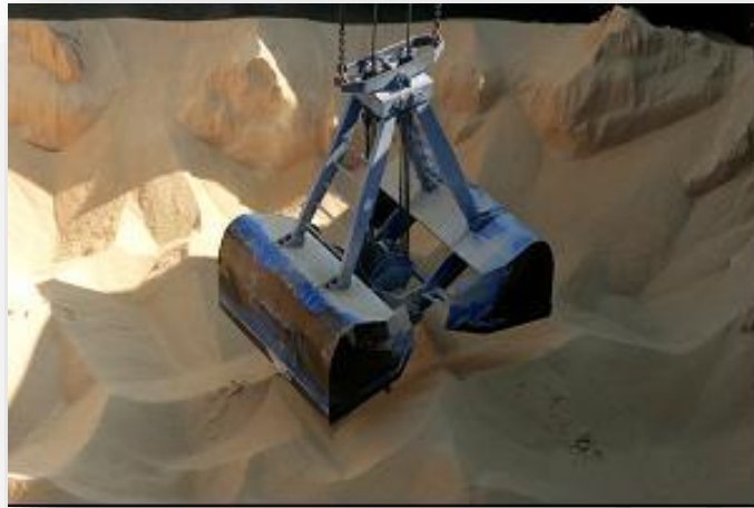
Systems must be in place to keep personnel away from grabs during hold operations
