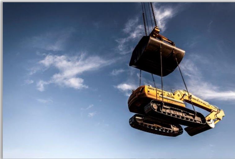
An excavator slung under a bulk grab.
