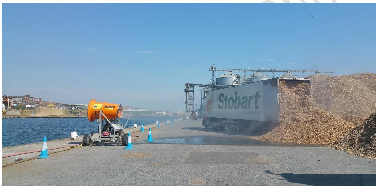
Examples of dust suppression using water sprays
