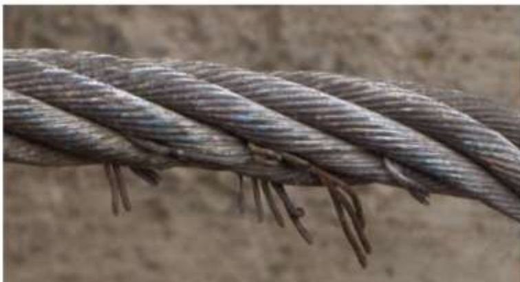
Fig 2: Spraggs [WIRE ROPES IN THIS CONDITION SHOULD NOT BE USED]
