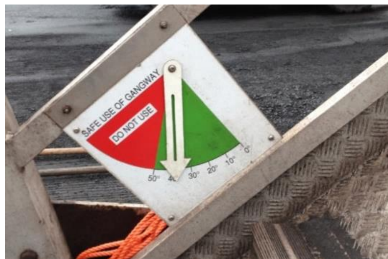
Figure 3 - An example of maximum design angle of use using an Inclinometer on a gangway
