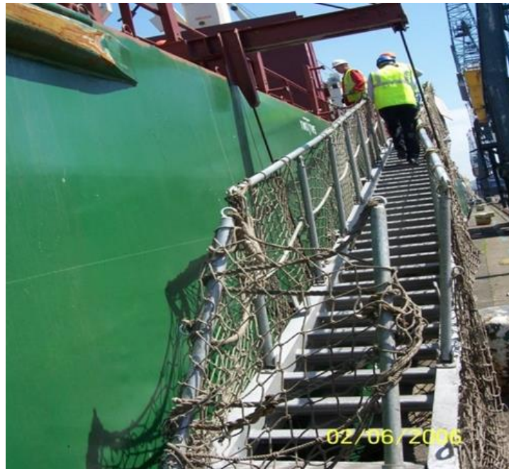
Figure 2 - Accommodation ladder with safety nets deployed
