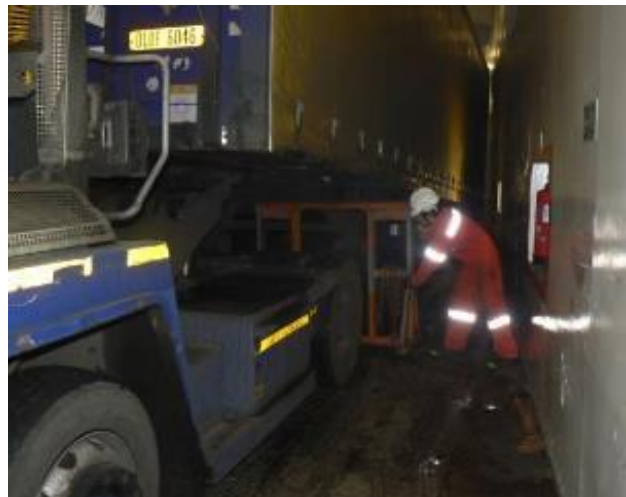
Figure 2. A traditional trestle being positioned
