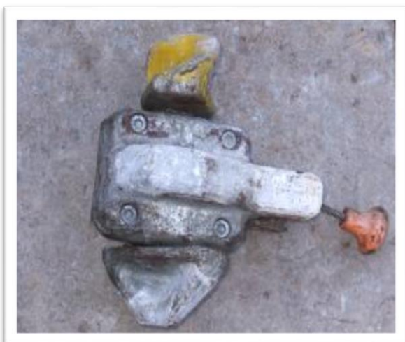
Single toggle semi-automatic twistlock
