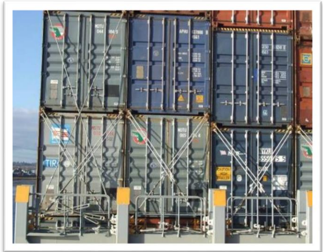
Lashing arrangement – double lashing with one high bars and three high bars in outboard cell
