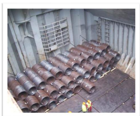
Wire Rod in Coil Loaded against a Swedged Bulkhead
