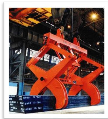
Duplex slab handling
