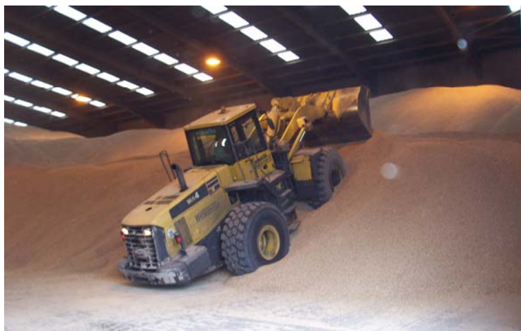
Figure 2 – Loading shovel working on cargo in a bulk shed
